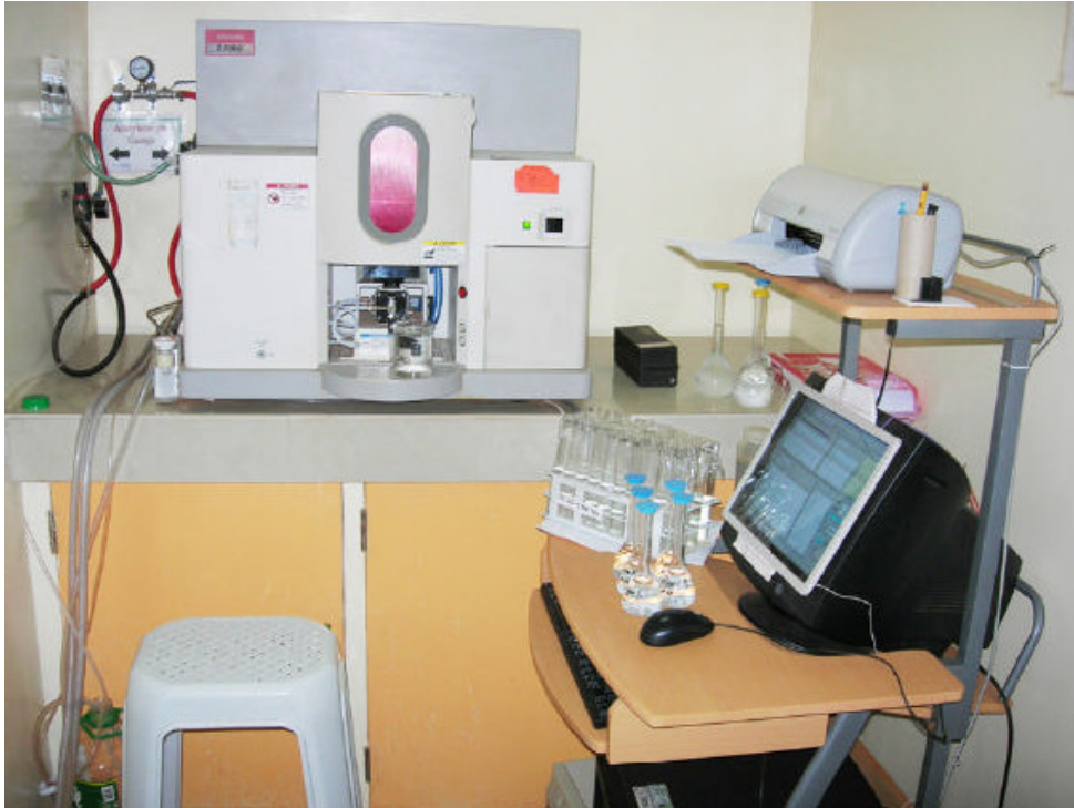
Figure 47: Hitachi AAS Unit in Ostrea Laboratory – NNMDC Compound.
