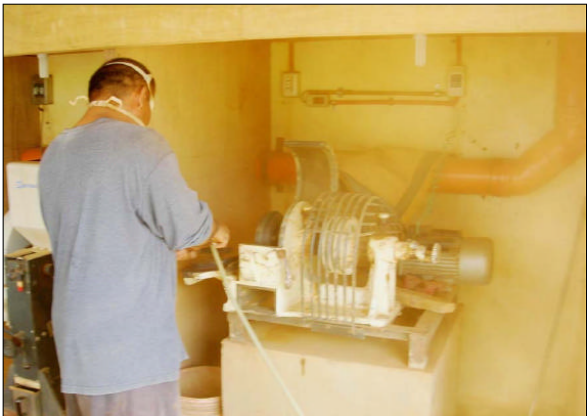
Figure 12: 'Bico' Final-Stage Pulveriser Unit in Operation – Ostrea laboratory – NNMDC Compound
